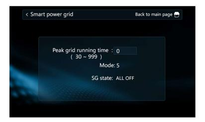
When there is neither SG signal nor EVU signal, you can set the maximum operating time of the unit and then turn off the unit.
