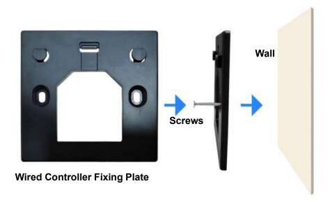
②Fasten the wired controller onto the fixing plate from top to bottom.
