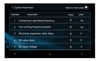
When unit in cascade mode, touch " System Parameters " and select the units you want to view. Grey means the unit is not connected.
